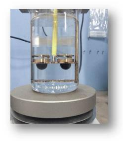
Degree of penetration of StarPatch: 250 dmm
