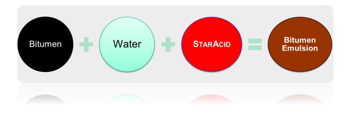
The additives called StarAcid and StarBas, depending on the type of bituminous emulsion that you want to produce, whether cationic or anionic respectively, are specially used in complex formulations studied in the Star Asphalt laboratories for the production of perfectly plastic and cold workable mixes.
