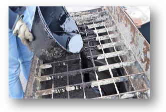
Ricicla is a bituminous binder for the reuse of road milling at room temperature. Its particular composition allows the following functions to be carried out against the old bitumen present in the milled material: wetting, regenerating, antioxidant and plasticizer. It is used for the "cold" production of plastic asphalt mix using 100% of milled material (RAP).
