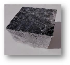
An exclusive feature of the asphalt mix obtained using this stick is the opaque aspect, almost dry, at the end of the production process, indicating a perfectly stable bond inert / binder, this is a prerequisite for the durability of the repaired deteriorated road surface, with a consequent energy saving, resources and money. Moreover, the opacity characterizing this type of asphalt allows not to grease or dirty means of transport
