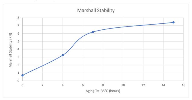
Marshall stability of the asphalt mix after aging – UNI EN 12697-34
