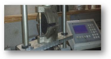
according to the results of the SHRP project, it simulates some months of curing asphalt mix in a hope under traffic, quantifiable in about 6 months of light traffic or 2 months of heavy traffic. To simulate shorter periods, intermediate tests were carried out. In particular, tests were carried out on freshly compacted specimens and specimens cured for 4h and 7h, with the aim to evaluate the material for shorter application periods behavior.
