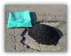
type of bitumen used. Normally the dosage varies from 15.00% to 35.00% on the weight of the bitumen.
