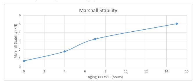
Marshall stability of the asphalt mix after aging – UNI EN 12697-34
