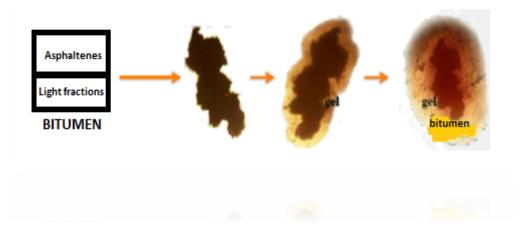
The conjugated effect of the high temperature and the presence of aromatic oils, as well as of resins, in the bitumen, allows the swelling of the rubber particles, which also come to duplicate their volume generating a bitumen-rubber gel: the additive binder, from lumpy becomes homogeneous and fluid.
