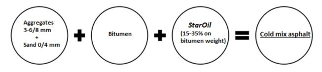
The additives called StarOil<sup>®</sup> are specially formulated for the production of cold plastic mix asphalt, performing the dual function of fluxing and plasticizing. They are not of oil origin but derive from renewable sources of plant origin.
